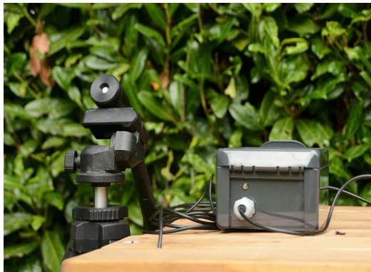
Remote Microphone and IP67 enclosure : A crude submersion test.
