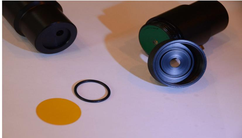
A disc of Kapton film is held against the o'ring inside the microphone front end. It is further sealed against water ingress with automotive instant gasket. A little axle grease is applied to the microphone front end thread to further discourage any seepage of water via the thread. This renders the front end waterproof.
