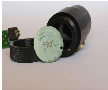
Showing the internal assembly left, and right note the alignment pin on the microphone housing, this locates with the hole in the mic disc.
