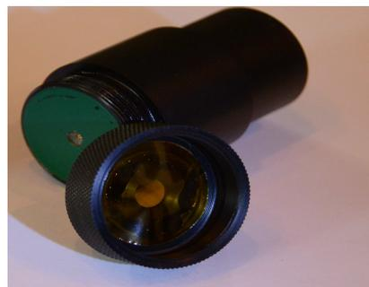
At the back end of the mic the connection is via a 3.5mm jack socket. This is not waterproof to a high IP rating, however water tends to run off at the back of the mic due to a turned ledge. Users can try a little instant gasket to discourage seepage around the jack if required. Although a jack plug connection might seem to be a poor choice of connector ( there are IP67-IP68 connectors available ) , it is chosen as it makes a low cost commonly available cable for the user.
